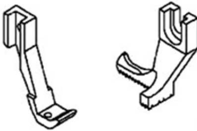
Wider feeding foot, toe on left side 較闊內壓腳，趾在左面
